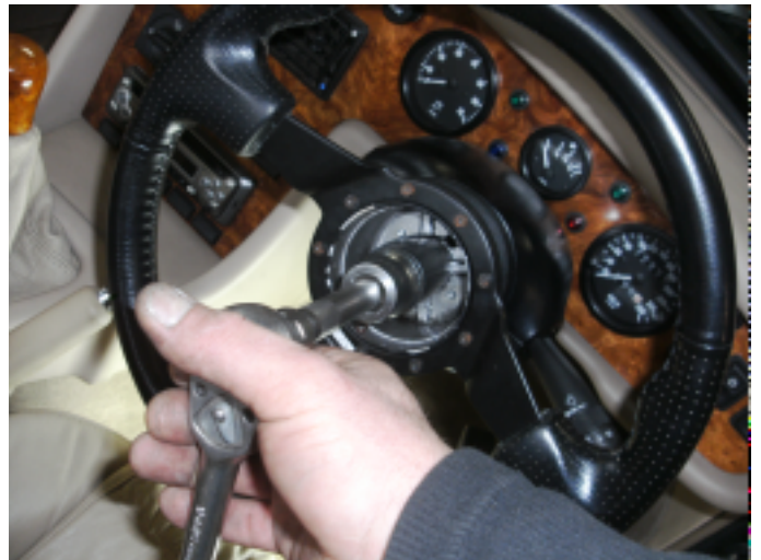
3.3 Removing steering wheel
