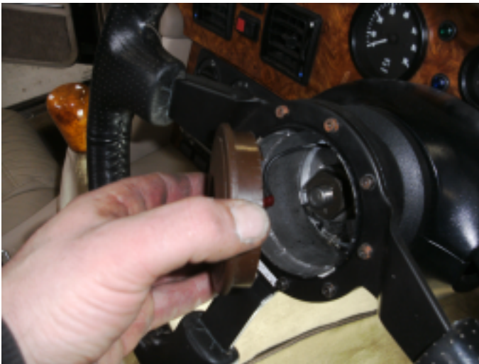
3.2 Removing horn button...
