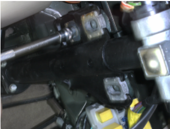
7.1 Removing bolts in mounting bracket
