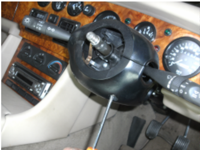
4.1 Removing stalk unit cover
