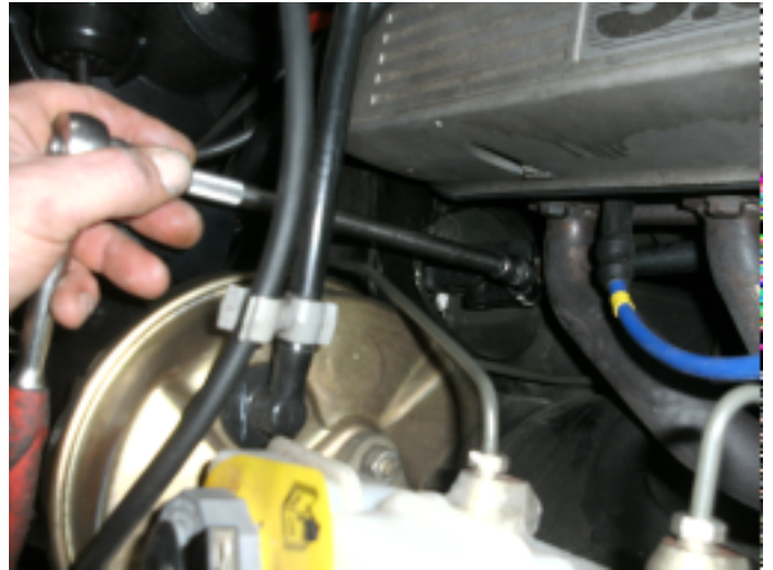
6.1 Undoing bolt in universal joint
