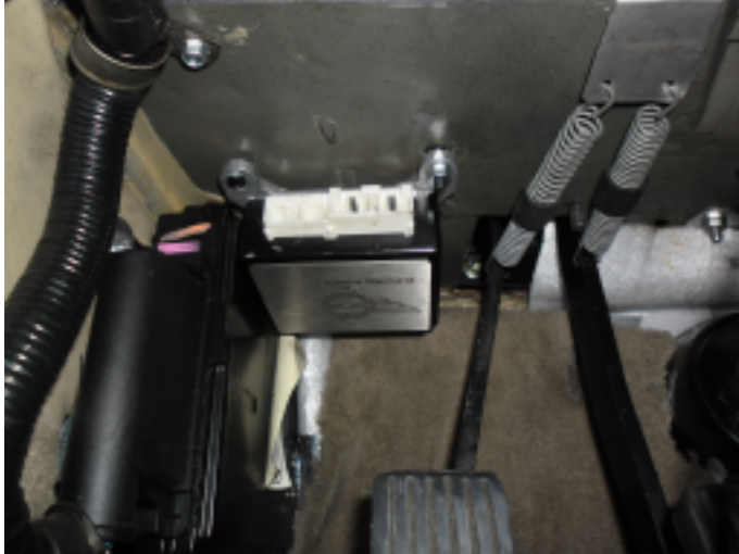
12.1. ECU installed underneath dashbord
